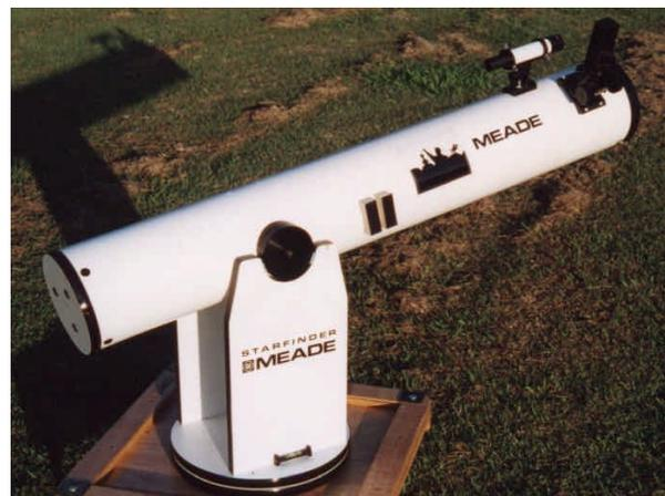
Newtonian telescope on Dobsonian mount.
