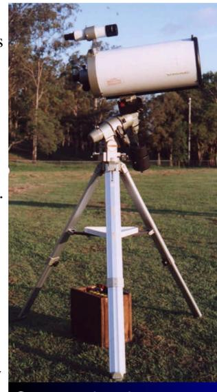
Cassegrain telescope on equatorial mount.
