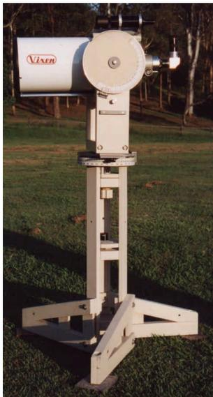
Cassegrain telescope on alt-azimuth mount.
