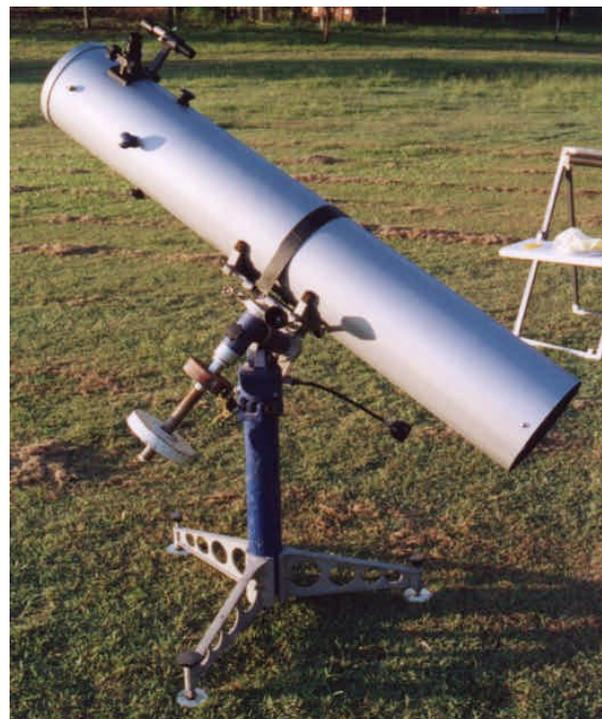
Newtonian telescope on equatorial mount.
